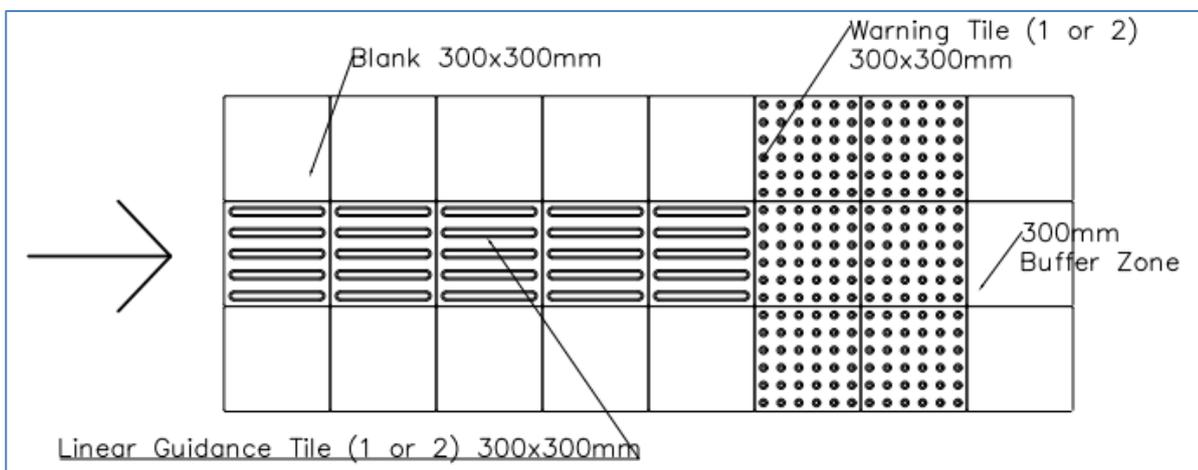
Fig. 5. General Testing Configuration [8]
