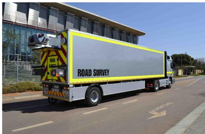
Figure 6 The MX8 and Waylink systems together with the Doppler Deflection system makes this a one of a kind TSD
