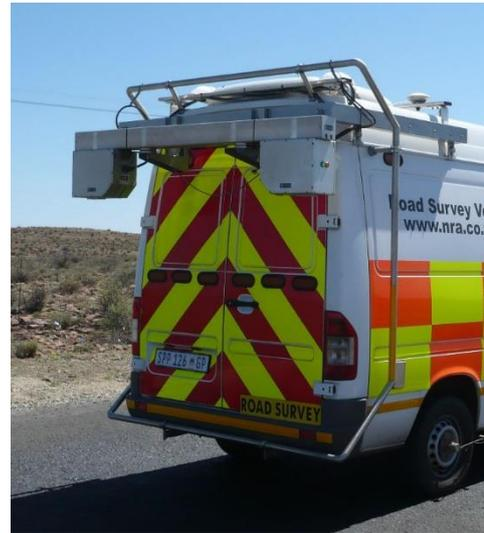
*Figure 4 The Waylink Crack detection system used infrared lasers for its light source*
