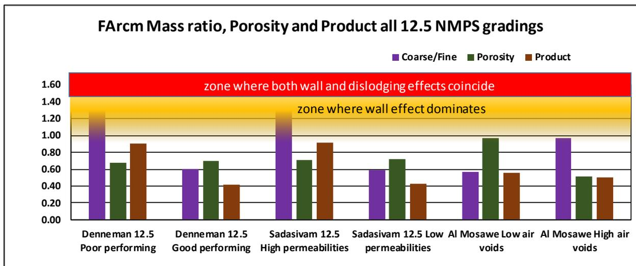
Figure 7: SCS to TCS fraction Ratio and Porosity and Product (Horak, et al., 2018)
