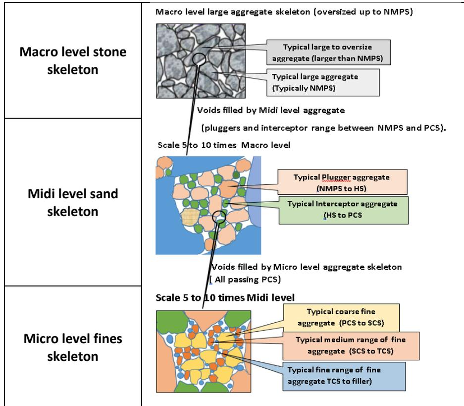
Figure 1. Illustration of Various Skeleton Infill Structures of Overall Aggregate Matrix.
