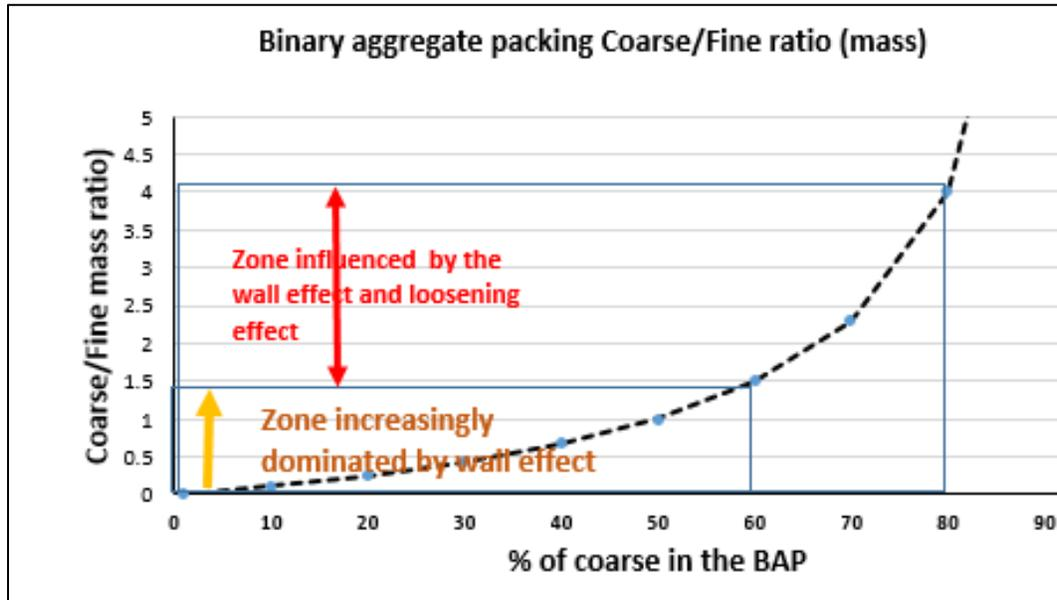
Figure 6: Coarse aggregate percentage versus the coarse/fine mass ratio of the BAP
