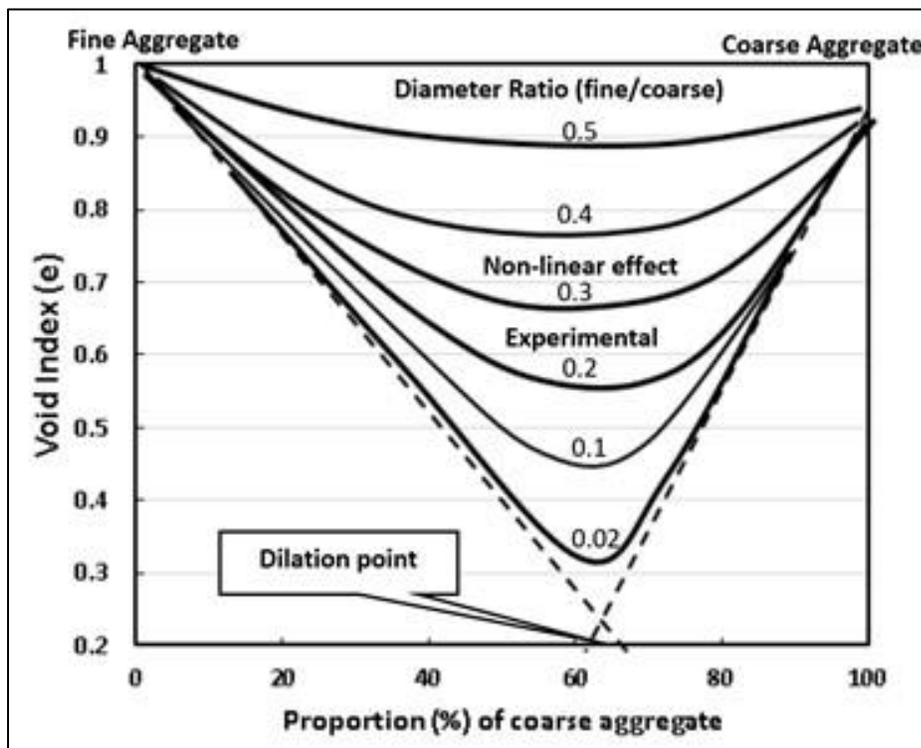
Figure 2: Typical Binary Aggregate Combination Porosity Influence with Varying Diameter Ratios and Proportion of Coarse Aggregate (Olard, 2011 based on Furnas, 1928)
