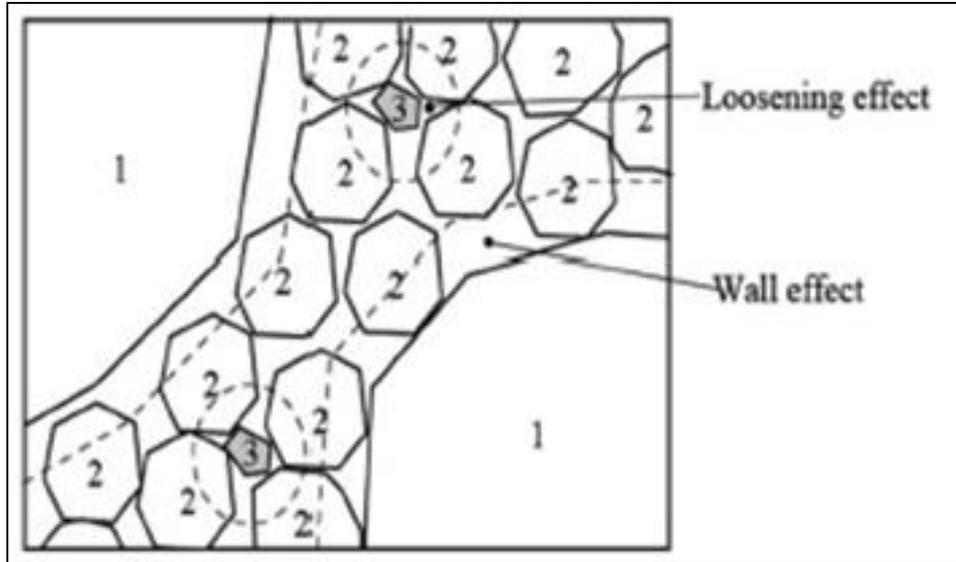
Figure 4: Schematic Illustration of Porosity Influence Due to the Wall and the Loosening Effect (Knop & Peled, 2016)
