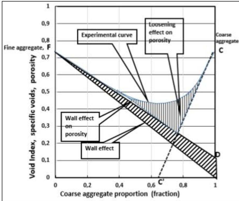
Figure 3: The Furnas Principles Applied to a Binary Combination of Coarse and Fine Aggregates (Olard, 2015)
