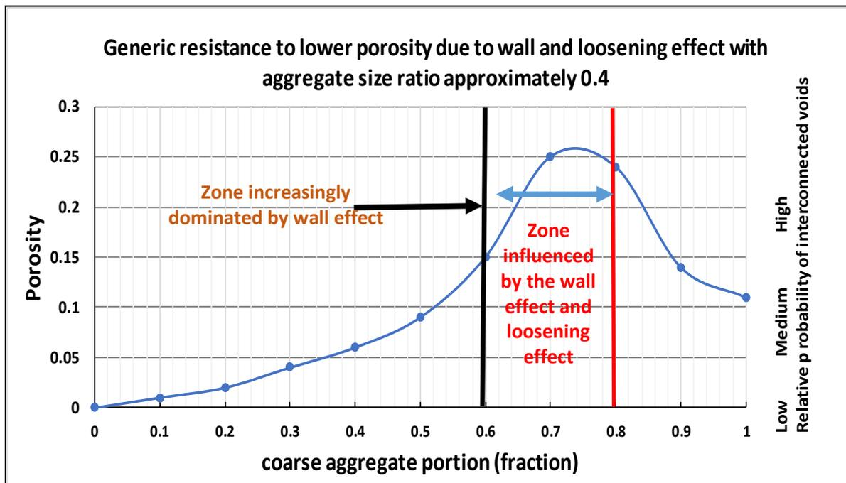
Figure 5: Resistance to Porosity Decrease Linked to the Effect of Coarse Aggregate Fraction in the Binary Mass Ratio and Associated Probability Effect on Interconnected Voids for a Typical Size Ratio
