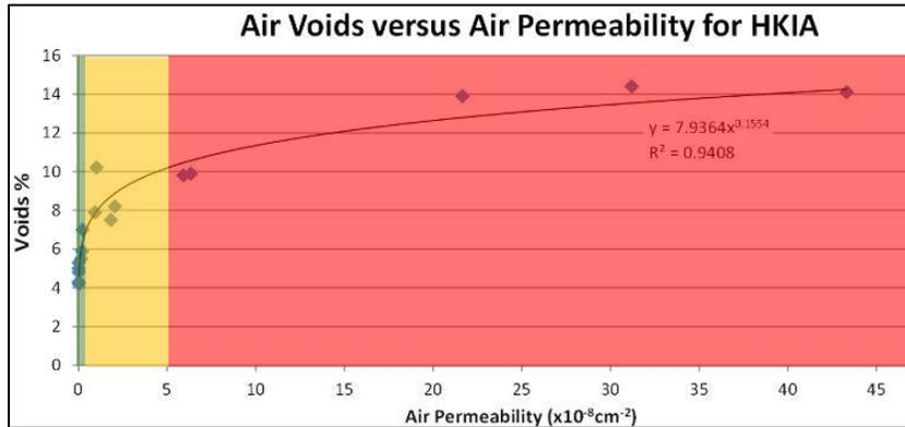
Figure 9: Air Permeability Versus Air Voids in the Mix on the Apron of HKIA (Horak, et al., 2012)
