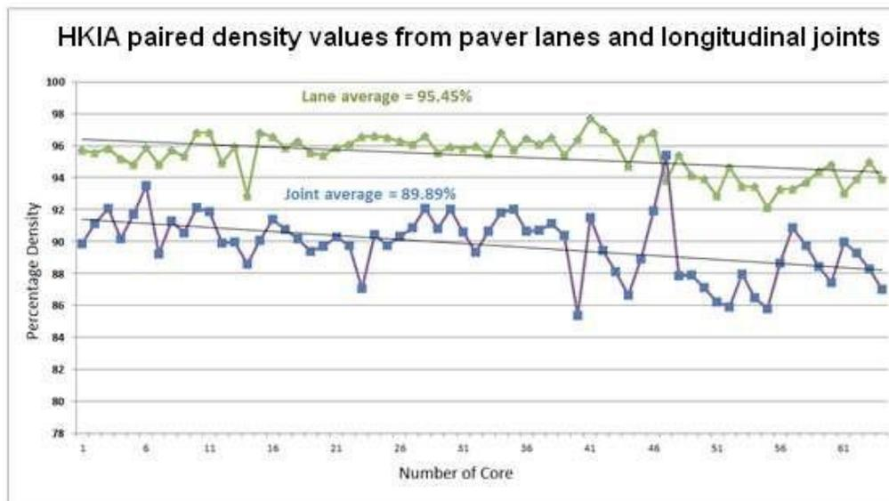
Figure 8: Paired Densities from Paver Lane and Joints on HKIA (Horak, et al., 2012)
