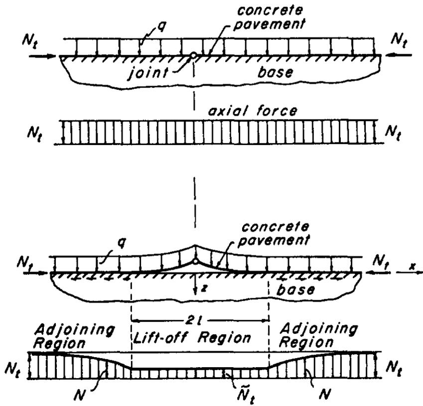
Figure 3: Axial forces in a concrete pavement after a blow-up [18]
