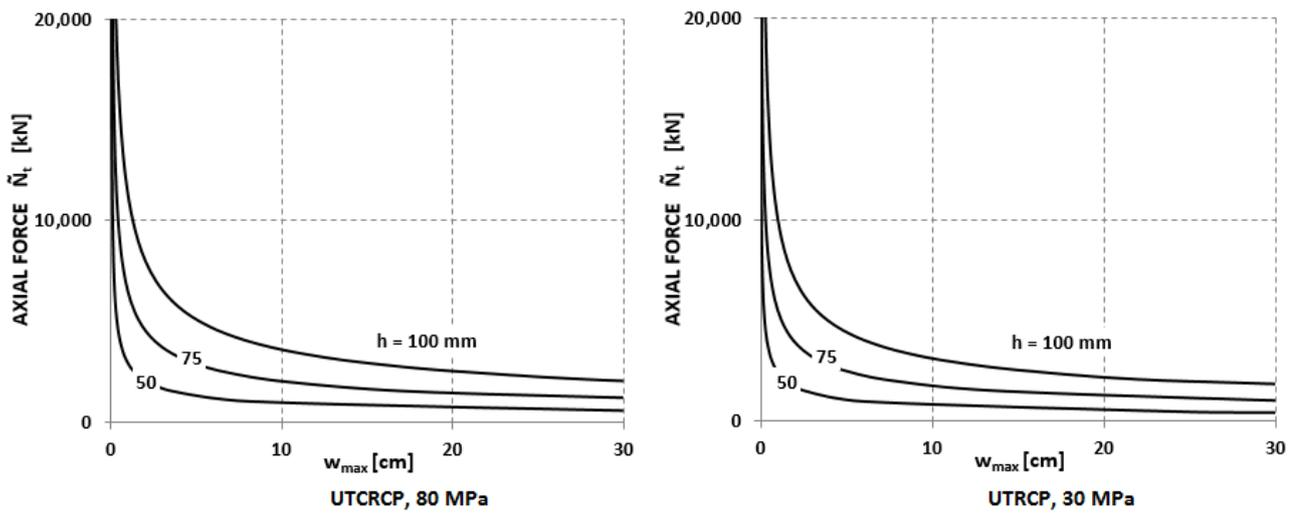
Figure 6: Axial forces,  $\tilde{N}_t$ , for UTCRCP and UTRCP with a joint/crack
