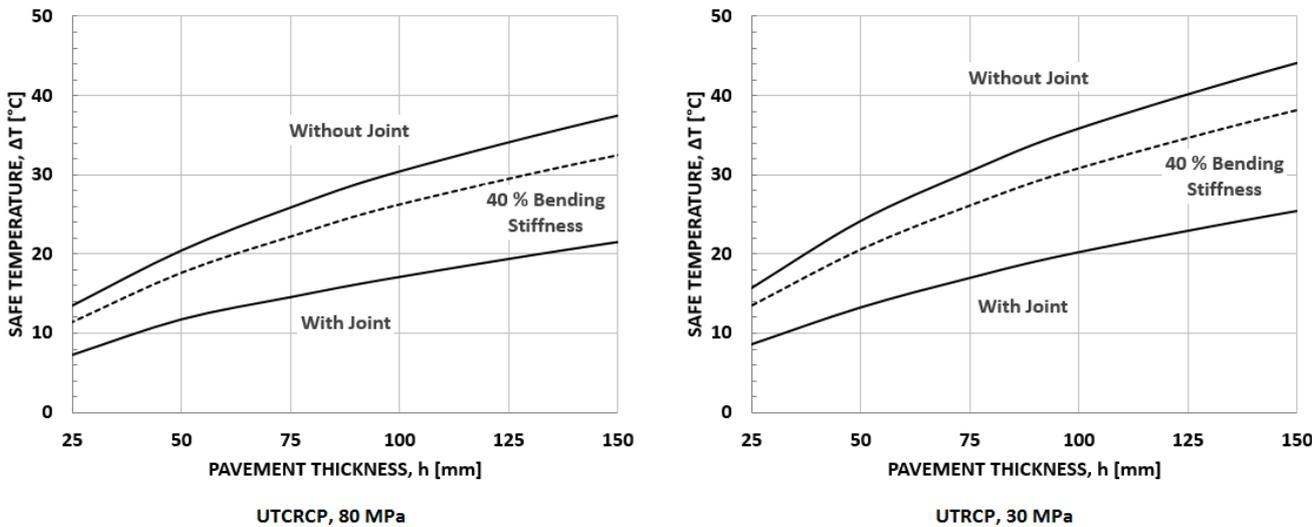
Figure 8: Pavement thickness influence on safe temperature increase
