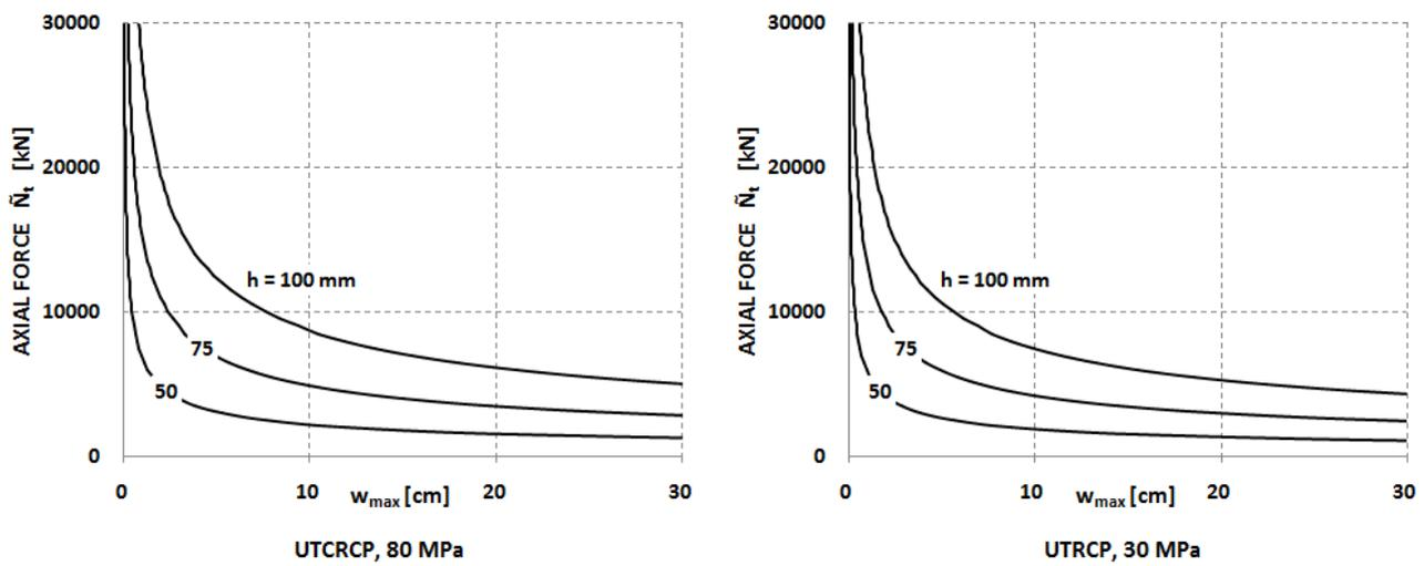
Figure 7: Axial forces,  $\tilde{N}_t$ , for UTCRCP and UTRCP without a joint/crack
