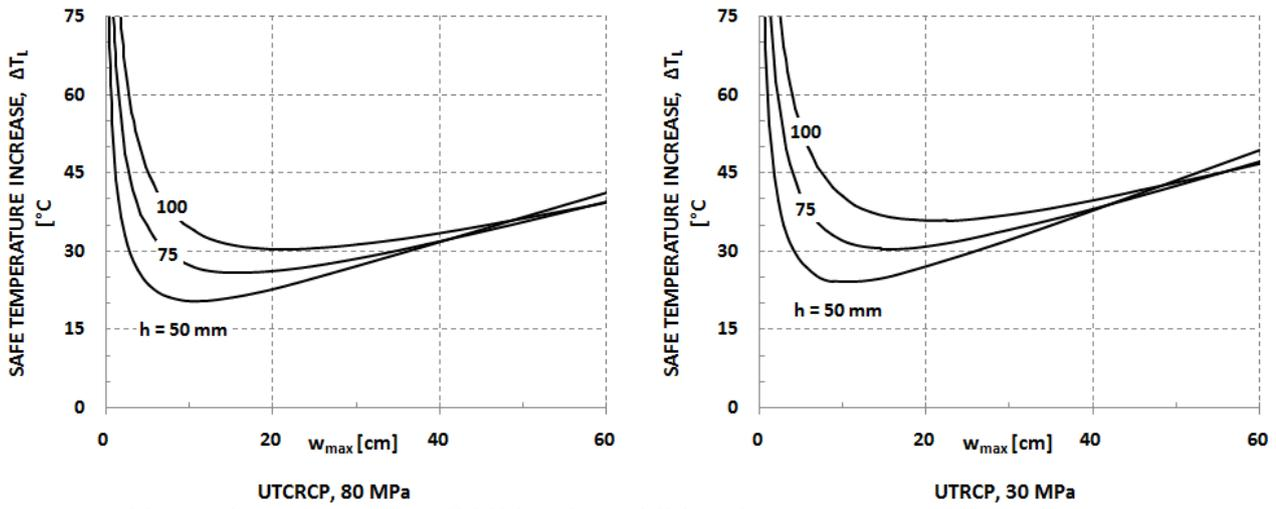
Figure 5: Equilibrium branches for UTCRCP and UTRCP without a joint/crack
