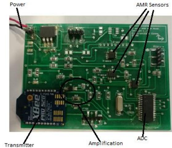
Figure 2 Fabricated sensor Node
