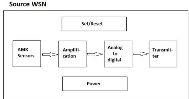
Figure 1 Sensor Node design
