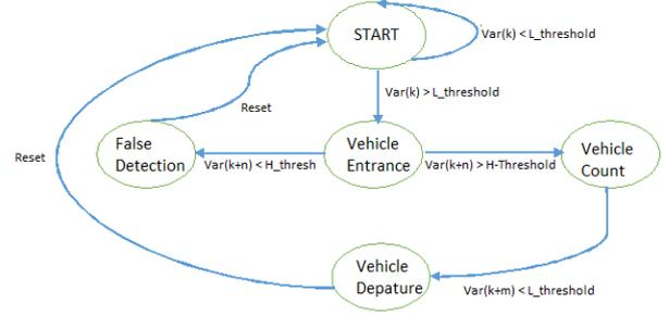
Figure 3 Vehicle detection state machine
