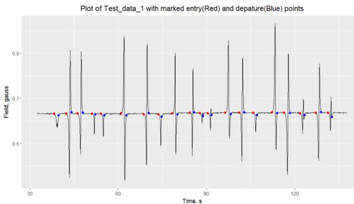
Figure 6 Magnetic signal with calculated entrance and departure points
